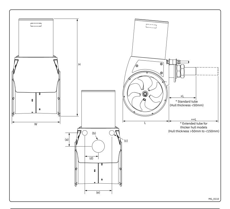
Thruster Measurements MC\_0239
