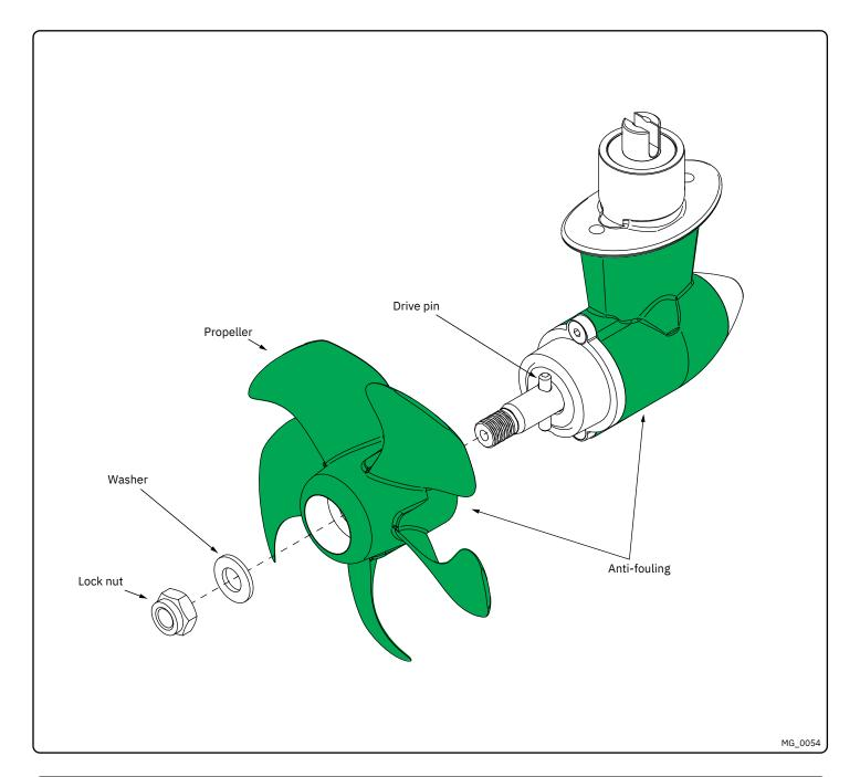
Propeller Installation MC\_0016
