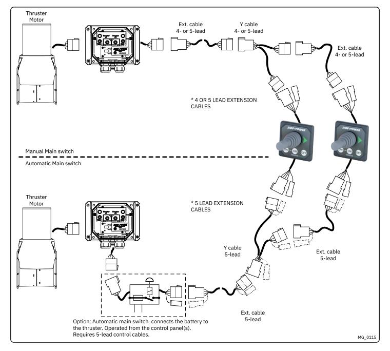
Control Panel Cable Installation MC\_0041
