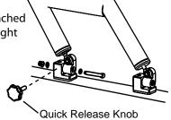
Attach lanyard from Quick Release Knob
