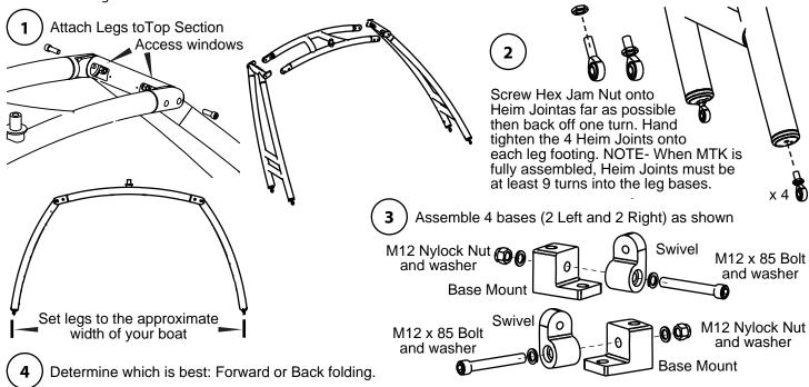
Make sure the legs are set to the approximate width of your boat. Forward folding is recommended if you will be adding speakers and board racks. Customer photos on our website can be helpful for mounting ideas and where to mount the tower.
