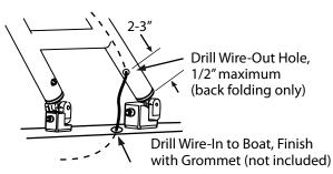
NOTE: You may conceal wires for speakers and other electrical accessories by adding wire in/out holes. Holes can be up to 1/2". Avoid solid areas inside your tower as shown to the right.
