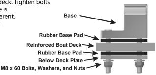
Component Stacking Through Reinforced Deck
